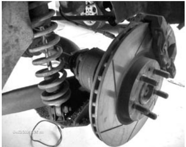
*A finished outboard conversion on a 75. The stock Dedion transaxle positions the brakes inboard where there is little air flow for cooling. The outboard system also allows you to run a larger rotor*
